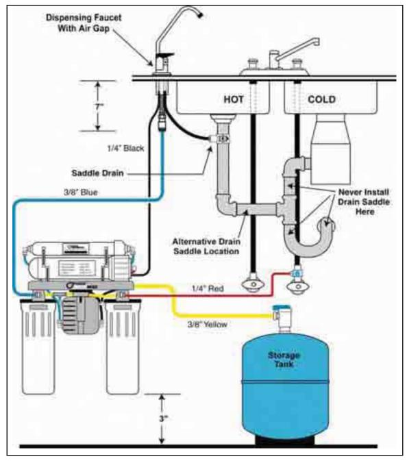
Figure 2: Installation Diagram
